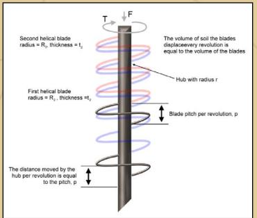
Figure 4.3 Helix Pier Installation Properties
